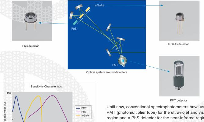
Until now, conventional spectrophotometers have used a PMT (photomultiplier tube) for the ultraviolet and visible region and a PbS detector for the near-infrared region. Neither detector, however, is very sensitive near the detector-switchover region. This prevents high sensitivity measurement in this range. The UV-3600 makes it possible to take high-sensitivity measurements in the switchover range by using an InGaAs detector.
