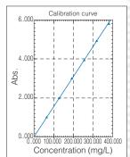
The figure on the far left shows spectra obtained by measuring aqueous KMnO4 solution at six concentration levels. A mesh filter was inserted on the reference-beam side and a differential method was used to perform measurement up to absorbance level 6. Using negative absorbance enables measurement with little noise, even at high absorbance levels. The figure on the near left shows the calibration curve for aqueous KMnO4 solution, and shows that linearity is maintained up to absorbance level 6.
