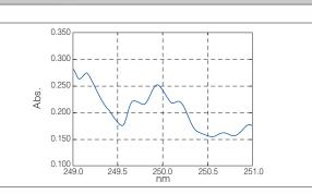
The spectrum shown on the left was obtained by enclosing benzene gas in a cell with an optical-path length of 10 mm and performing measurement. The spectral bandwidth is 0.1 nm. The triplet in the neighborhood of 250 nm (enlarged above) can be observed clearly. This instrument allows high-resolution spectra to be measured with little noise.
